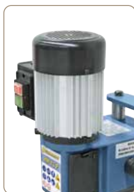
Motor de aluminiu puternic conform IP 54
