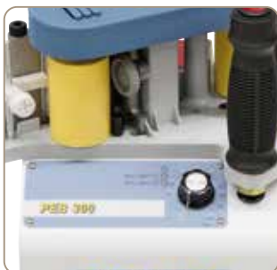
The required working temperature is set by potentiometers.
