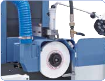
Manual parallel dressing device features micrometric adjustment as standard.
