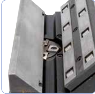
Includes milling head with commercial HM-reversible plates.
