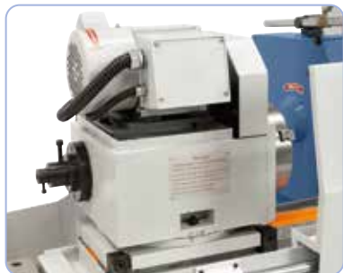
Spindle head tilts from 0° - 90° for conical grinding operations.
