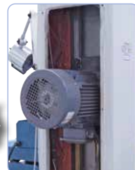
The solid guiding of the grinding head ensures precise infeed.
