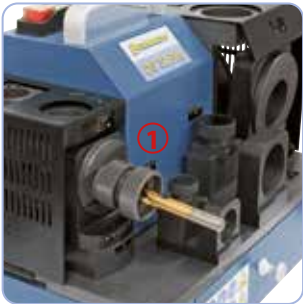
1. Grinding the point angle \varnothing 2 - 13 mm
