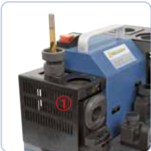
1. Relief-grinding of the relief angle \varnothing 2 - 13 mm
