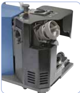
Grinding of the relief angle at 2-edged end mill
