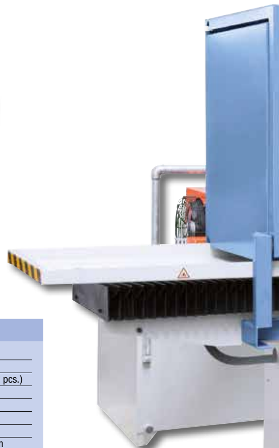
Coolant device with extractor, magnetic separator and paper filter are optionally available.
