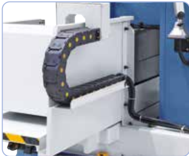
Including cable guiding by energy chain
