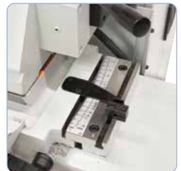
For conical grinding between the centers the table can be tilted from +3° bis -7°.
