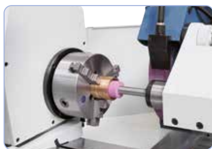
Comes complete with removable internal grinding device.
