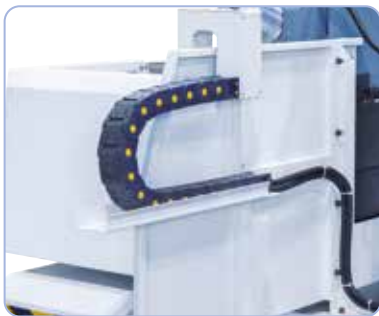
Including cable guiding by energy chain
