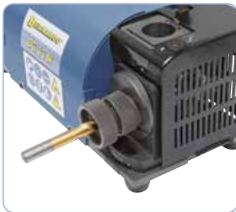
Grinding the point angle
