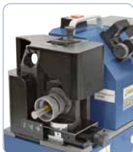
Grinding the point angle
