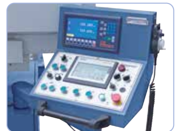
Clearly arranged control elements at the tiltable control panel
