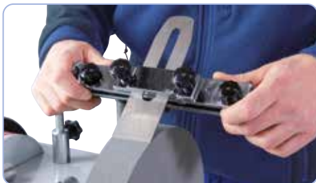
05-2054 Plane camper jig: Suitable for plane irons and chisels with a maximum width of 70 mm and maximum thickness of 6.5 mm
