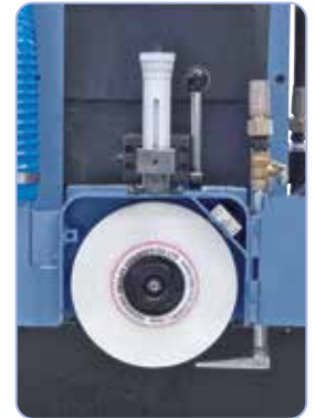
The spindle features pre-tensioned bearings to ensure high accuracy and a smooth run.
