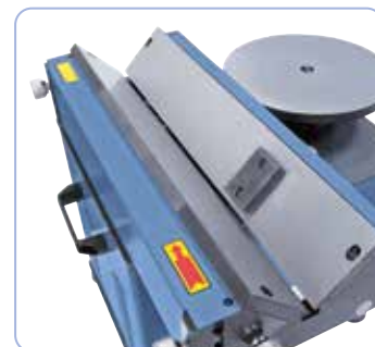
Grounded guide rail with workpiece fence.
