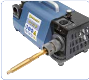
Grinding the point angle
