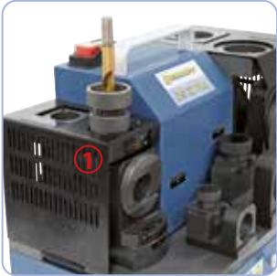
1. Thinning \varnothing 2 - 13 mm / 2. Thinning \varnothing 8 - 32 mm
