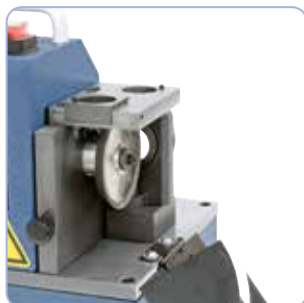
Diamond grinding wheel SDC comes standard
