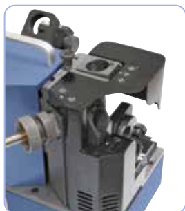
Grinding of the relief-angle at 3- or 4-edged end mill
