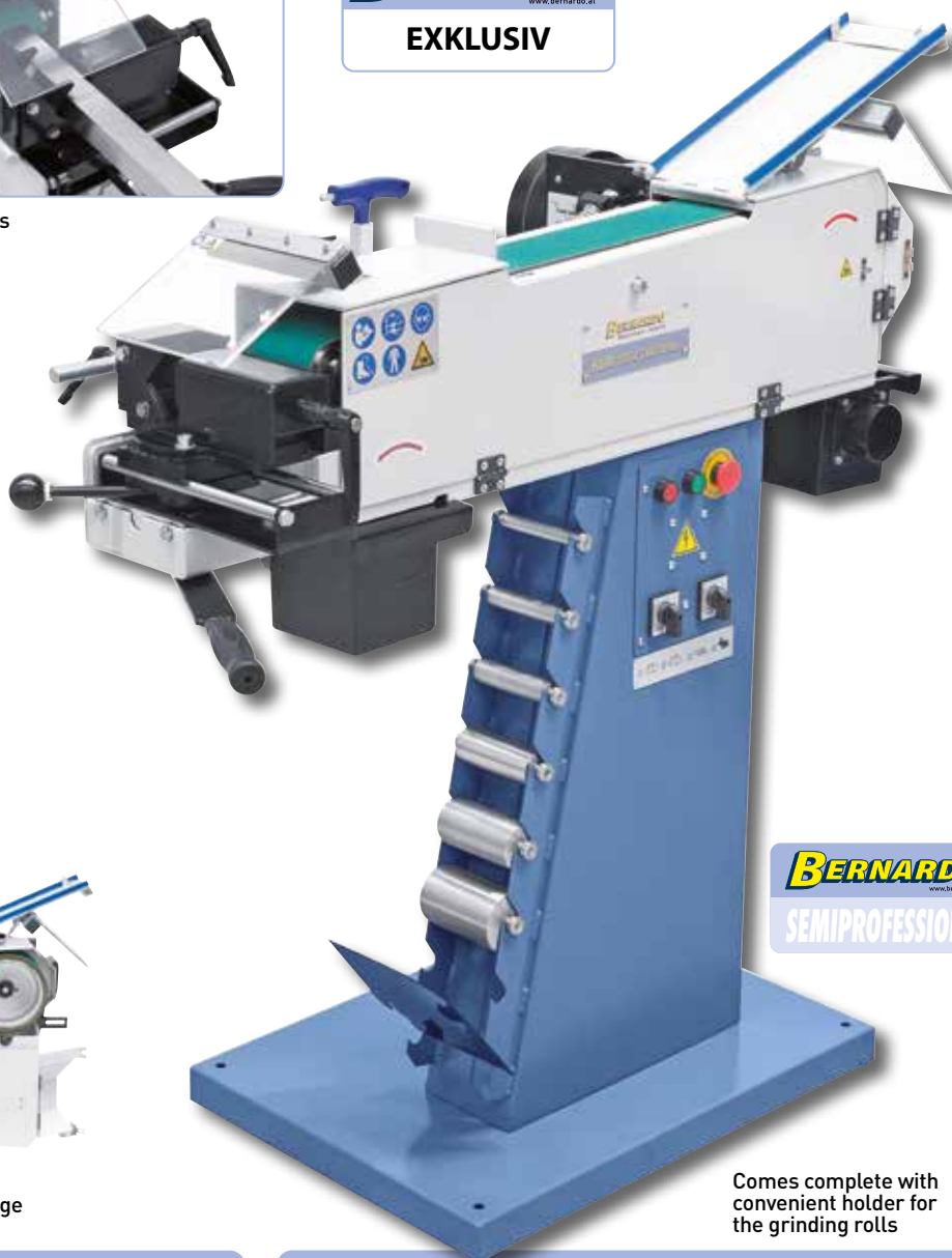
Universal vice allows clamping of pipes and profiles
