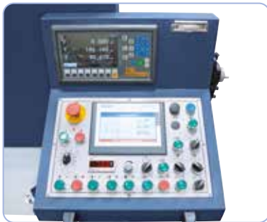
Including Siemens SMART-Panel IE V3 with touchscreen and electronic handwheel
