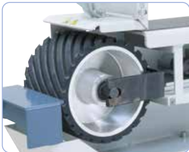
Contact disc 70° - 74° Shore A, ideal for roughing.
