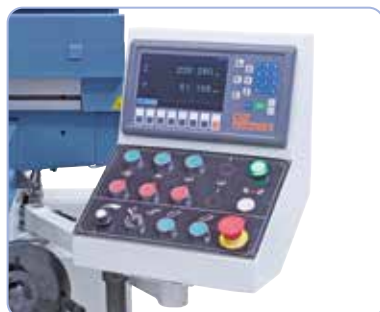
Clearly arranged control elements at the tiltable control panel
