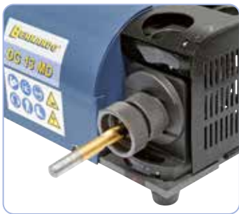
Grinding the point angle
