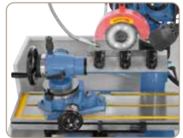
Sharpening of cutter knives.
