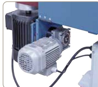
Sanding belt oscillation with independent motor.
