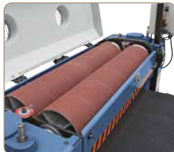
2 sanding rollers for rough and fine grinding in one pass.
