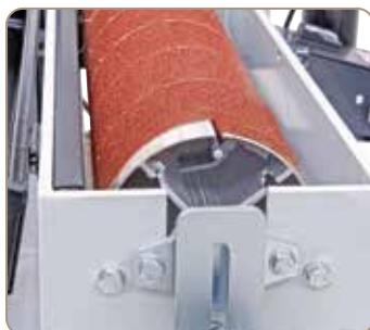
Quick clamp system for sanding belt.
