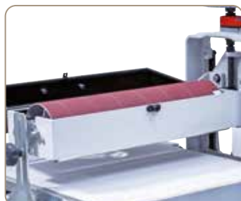
Lift dust hood to change the sanding belt.
