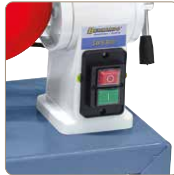
On-/Off-switch in accordance with IP 54 standards and undervoltage release.
