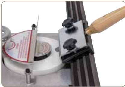
Grinding of carving knife
