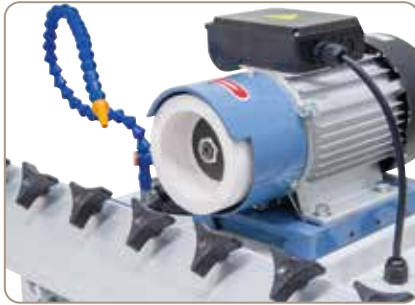
User-friendly clamping system for cutter knife.
