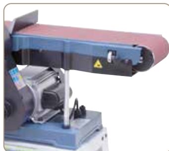
Large face sanding area with workpiece fence.
