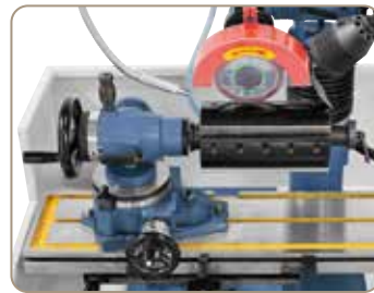
Sharpening of cutter block.
