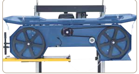
Tiltable covers allow for easy bandsaw blade change.
