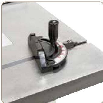
The serially mitre fence is adjustable from -60^{\circ} up to +60^{\circ} and will be guided in the T-slot of the table
