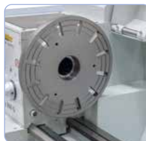
For clamping of irregular shaped workpieces, the machine can be equipped with a 250 mm face plate.
