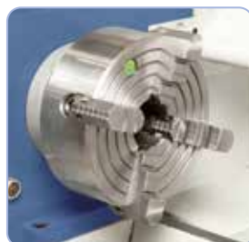
4-jaw independent chuck 200 mm with reversible jaws comes standard.
