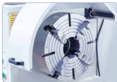
Independent chuck 400 mm for clamping of irregular shaped workpieces. (optional)
