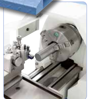
3-jaw chuck 125 mm includes hard inside and hard outside solid jaws.
