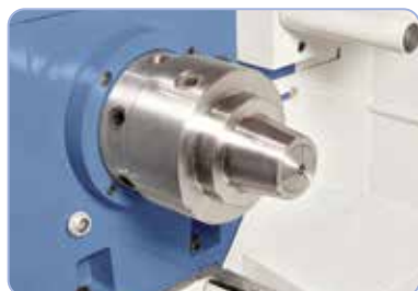
Optionally available: 5C fixture, clamping area 3 - 26 mm
