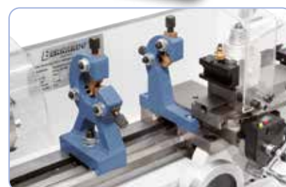
Using the rests allows easy processing of long workpieces.
