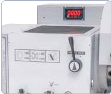
Electronic, stepless speed adjustment, digital display allows easy readout.
