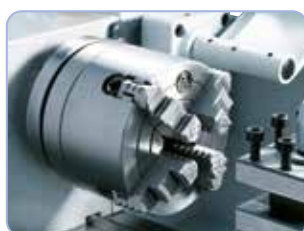
Independent chuck 100 mm ideal for clamping of asymmetric workpieces (optional)
