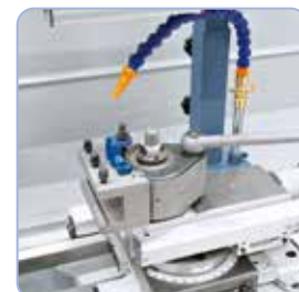
The machine can be equipped with a quick change tool post holder to raise efficiency.
