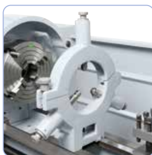
Steady rest to support long and thin workpieces.
