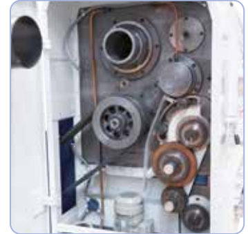
The hardened main spindle with 130 mm spindle bore is bedded on tapered roller bearings and radial roller bearing.
