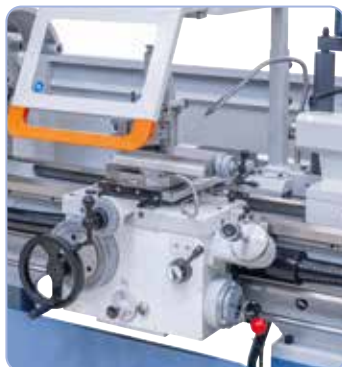
42 freely adjustable feeds are available for the longitudinal and cross travel of the apron and the top support.
