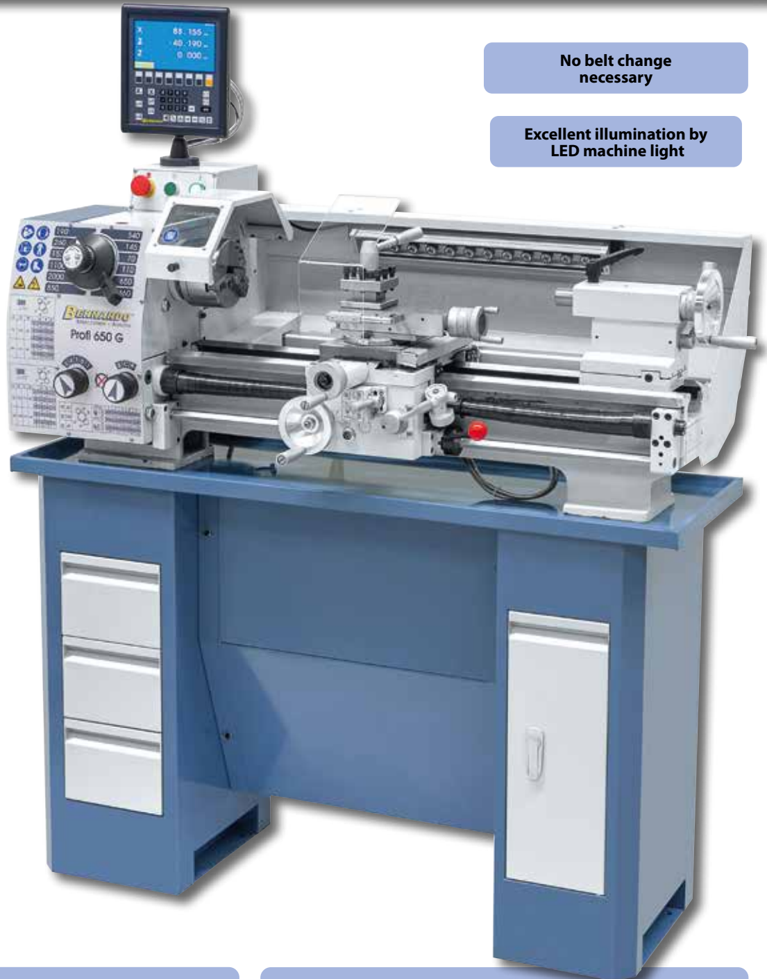
The tailstock with one-hand clamping can be moved for taper turning and is optionally available with a ball nose live center
