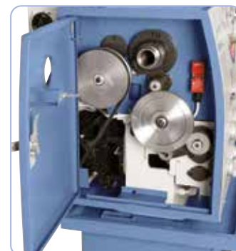
Standard accessories include change gears for thread cutting.
