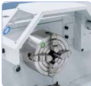
Independent chuck (optional accessory) allows clamping of irregular shaped workpieces.
