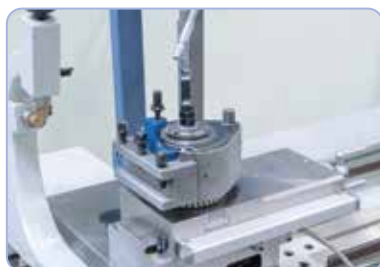
The machine is equipped with a quick change tool post holder to raise efficiency.
