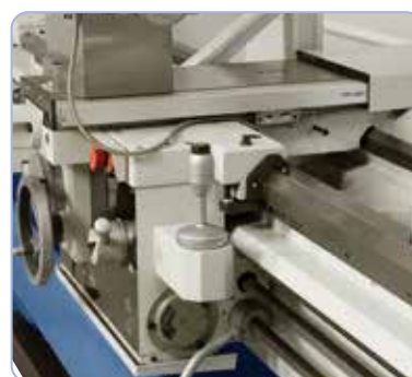
Complete with rapid feed for longitudinal and cross travel of apron
