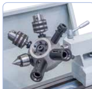
Machine can be equipped with revolving tailstock turret for economic operating
