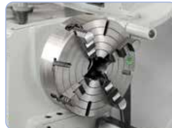
Independent chuck 320 mm for clamping of irregular shaped workpieces. (optional)
