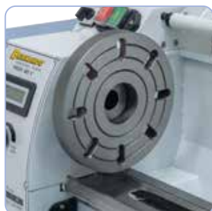
Face plate (170 mm) to clamp irregular shaped workpieces available at request.
