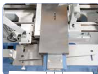
Taper turning attachment optional available, turning length 455 mm, setting angle +/- 8°.
