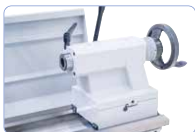
The solid tailstock with spindle taper MT 4 can be adjusted for taper turning.
