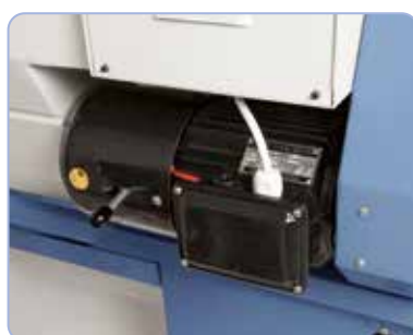
Powerful motor with magnetic brake in accordance with CE-standards.
