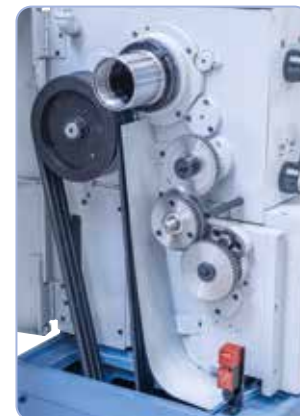
Hardened main spindle with precision taper bearing for high concentricity, teething Opti-belt-V-belt for optimal power transmission.
