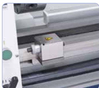
Micrometer longitudinal fence and safety clutch are part of standard equipment.
