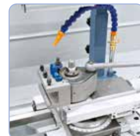
The machine can be equipped with a quick change tool post holder to raise efficiency.
