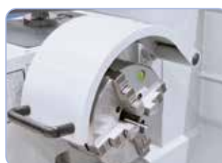
4-jaw chuck 160 mm allows centric clamping of square sections (optional)
