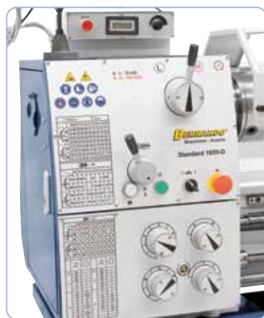
Convenient controls, all switches and control elements are clearly arranged on gear head.
