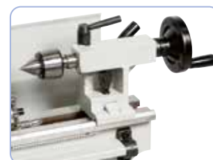
Tailstock (MT 2) can be adjusted for taper turning.
