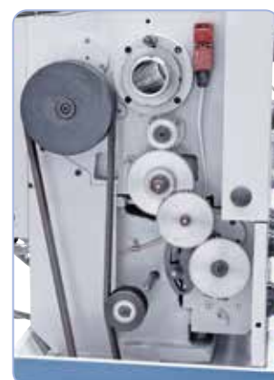
Serially equipped with change gears for thread cutting.
