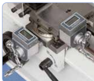
Serially equipped with digital display to ensure precise feed and readout when turning.
