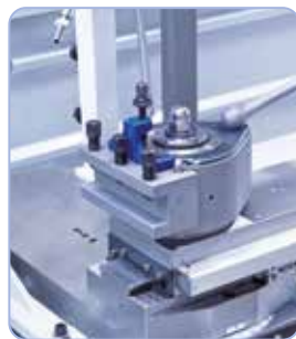
The machine is equipped with a quick change tool post holder to raise efficiency.
