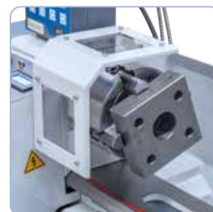
A 100 mm independent chuck is optionally available for clamping of irregular shaped workpieces.
