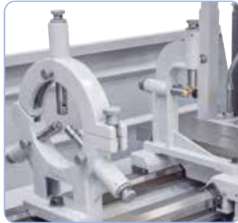
Complete with steady and follow rest to allow for solid support of long workpieces.
