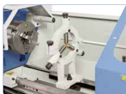
Steady rest with bronze guide to stabilize long workpieces.
