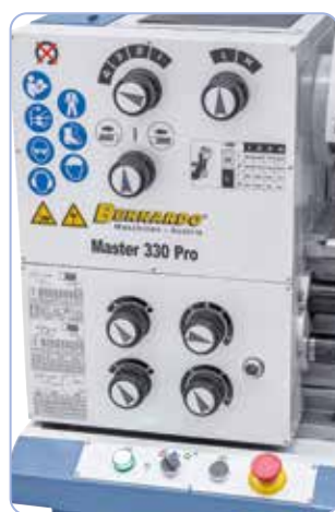
Ergonomically arranged control elements on gear head - hardened and polished gears allow for smooth run.
