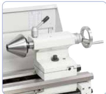
The tailstock with one-hand clamping can be moved for taper turning and is optionally available with a ball nose live center
