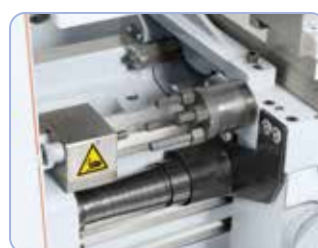
4 adjustable fence and micrometer longitudinal fence, ideal for serial works.
