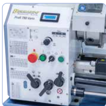
Electronic, stepless speed adjustment – easily read on digital display.
