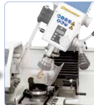
The tiltable mill head offers a variety of applications.
