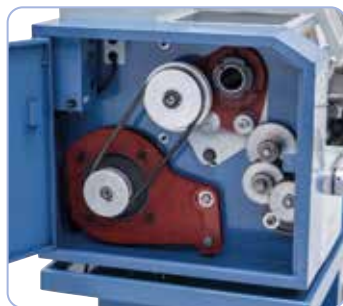
Serially equipped with change gears for thread cutting.
