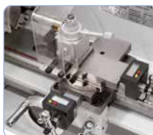
The machine is equipped with a quick change tool post holder to raise efficiency.
