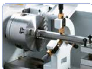
Steady rest with bronze guides to stabilize long workpieces
