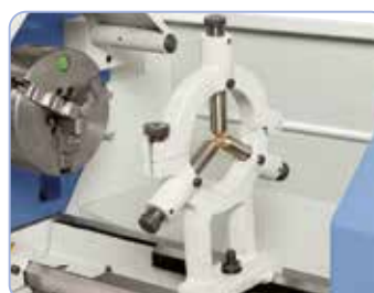
Steady rest with bronze guide to stabilize long workpieces.
