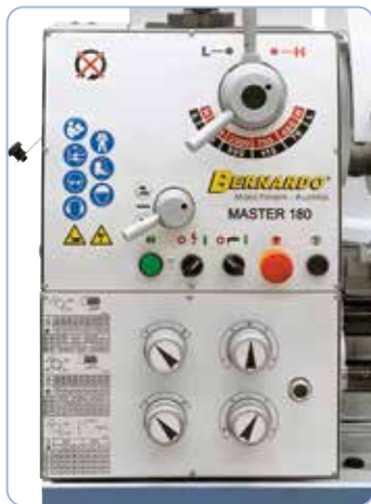
Straightforward feed and speed setting on gear head. Hardened and polished gear wheels saturated in oil ensure smooth operation.
