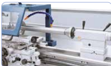
Ball nose live center 100 mm, ideal for clamping of pipes and hollow parts (optional).
