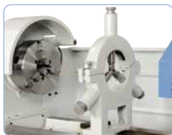
Steady rest with bronze guiding supports long workpieces up to diam. 180 mm.
