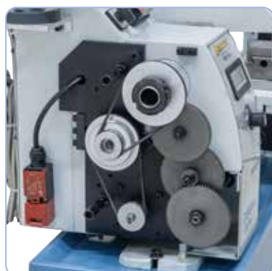
Complete with change gears for thread cutting.
