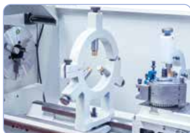
Steady rest with bronze guiding supports long workpieces
