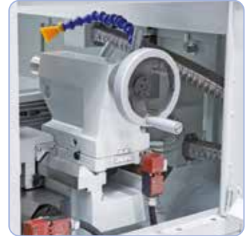
The solid tailstock with spindle taper MT 4 can be adjusted for taper turning.
