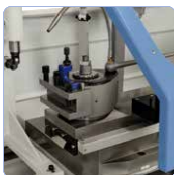
The quick change tool post holder allows a significant reduction of downtime and guarantees high repeat accuracy
