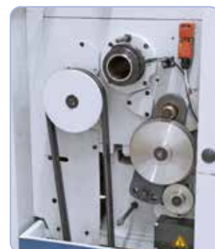
Standard accessories include change gears for thread cutting.
