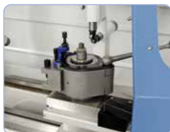
The quick change tool post holder allows a significant reduction of downtime and guarantees high repeat accuracy
