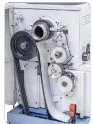
Hardened main spindle with precision taper bearing for high concentricity, teethed Opti-belt-V-belt for optimal power transmission.
