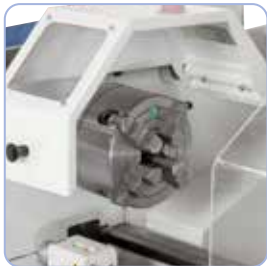
Independent chuck (optional accessory) allows clamping of irregular shaped workpieces.
