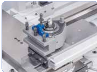
To raise efficiency the machine is equipped with a quick change tool post holder
