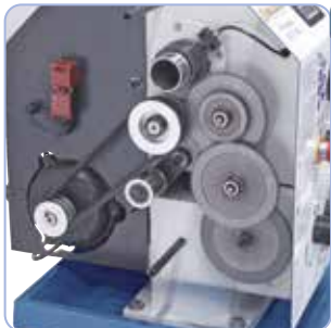
Hardened spindle, high-quality taper bearings ensure high concentricity of spindle nose ( \leq 0.009 mm)
