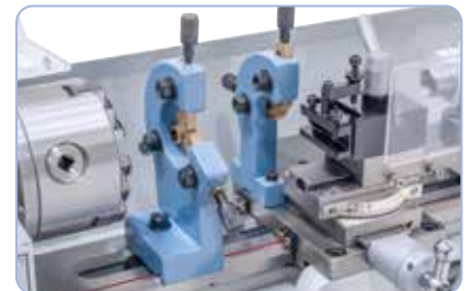
Using the rests allows easy processing of long workpieces.
