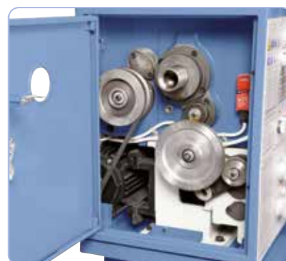
Change gears for thread cutting come standard.
