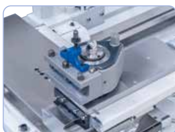
The 40 position tool post and holder set system Multifix raises efficiency and ensures a high repeat accuracy.
