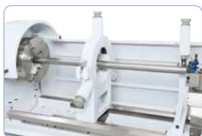
Serially equipped with steady rest for clamping of long workpieces.
