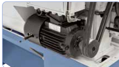
Powerful motor with magnetic brake in accordance with CE-standards.
