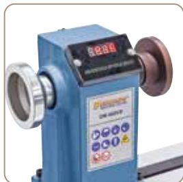
LED display allows for convenient speed readout.
