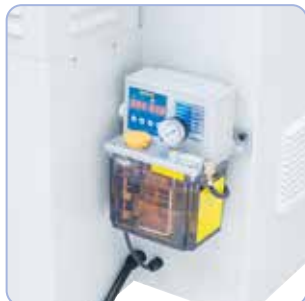
Electronic central lubrication comes standard
