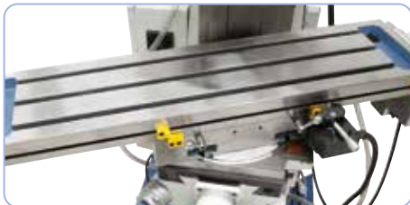
Milling table tilts from -45^{\circ} to +45^{\circ} .
