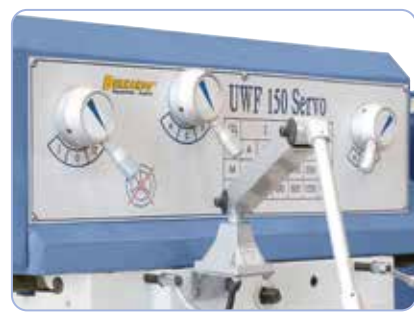
User-friendly control elements allow easy and quick speed change.
