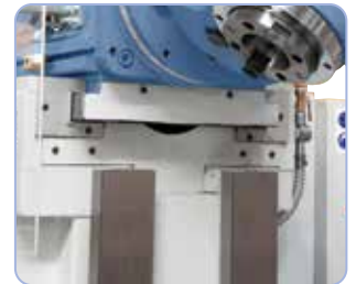
Large rectangular guides at the y- and z-axis guarantees an increase in stability (FU 1600 / FU 2000).
