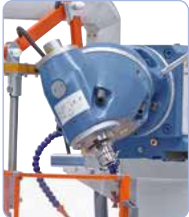
Universal mill head adjustable to various angles.
