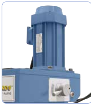
Reduction gearing allows for convenient pre-selection of gears, speed adjustment via potentiometer.
