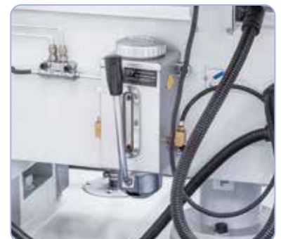
Central lubrication for x-, y- and z-axis comes standard.
