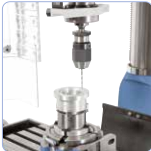
Drilling of coordinates
