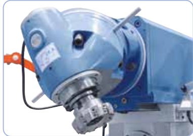
The adjustment of the 90° and 45° level allows the universal mill head to be set to various different angles.
