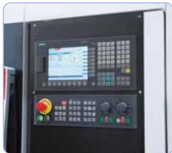
Comes standard with Siemens Sinumerik control with LCD color display for high efficiency and easy handling
