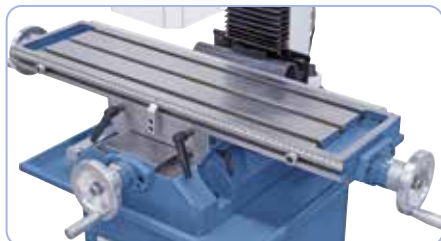
Surface treated cross table with 3 T-slots.
