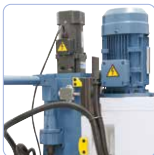
Lift motor for height adjustment of mill head comes included.
