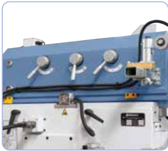
User-friendly control elements allow easy and quick speed change.
