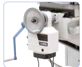
Comes complete with automatic table feed in y-axis.
