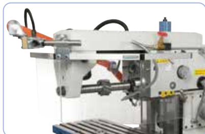
Horizontal milling with counter bearing.
