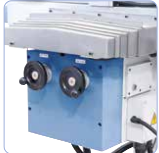
Electronic hand wheels for manual travel and 3 powerful servo motors in x-, y- and z-axis come standard.
