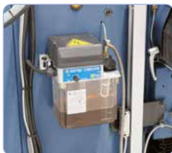
Electrical central lubrication for all guide rails and spindles
