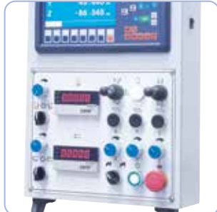
Quick and easy setting of the required feed speed directly at the control panel.
