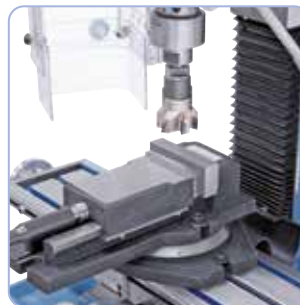
Milling with carbide indexable face milling cutter (Art. no. 42-1058)
