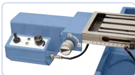
Optional with steplessly adjustable table feed for increased comfort FTV 9.
