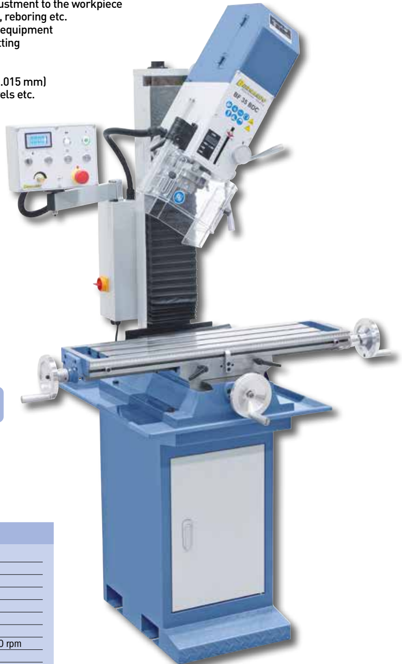
Digital speed and spindle stroke indicator included as standard equipment
