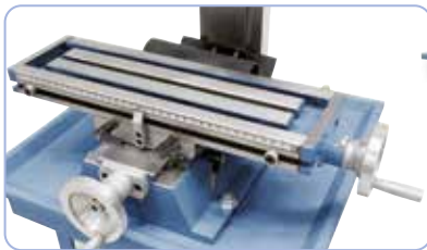
Surface treated cross table with 3 T-slots.
