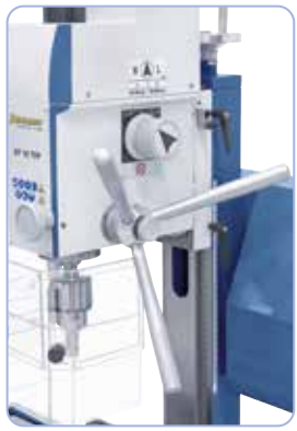
Large star handle allows easy spindle feed when drilling, handwheel allows fine adjustment when milling.
