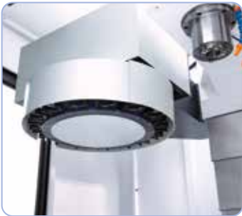
16-station tool changer for short changeover times
