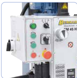
Ergonomically arranged control elements on the front of the machine.
