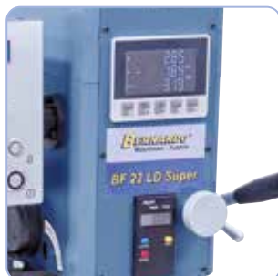
Serially: 3-axis digital readout
