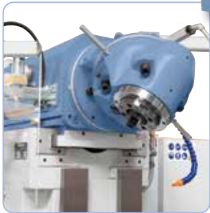
The adjustment of the 90° and 45° level allows the universal mill head to be set to various different angles.
