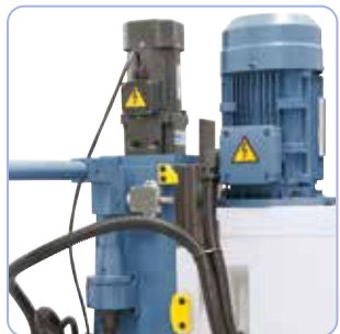
Lifting motor, as part of standard accessories, allows for convenient adjustment of mill head
