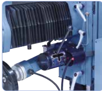
Selector lever for feed axis (picture for x- and z-axis), adjustment of the feed speed by potentiometer at the control panel.
