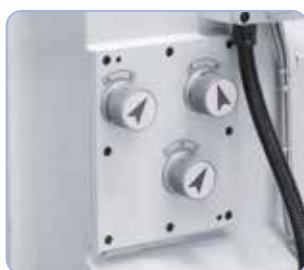
User-friendly gear controls for horizontal spindle come standard
