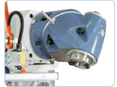
Universal mill head features 2 rotating axis, adjustable to various angles.
