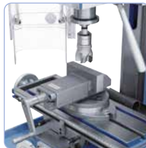
Milling with carbide indexable face milling cutter (Art. no. 42-1057)
