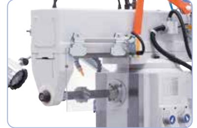
Complete with counter bearing and long milling arbor for milling in horizontal position.
