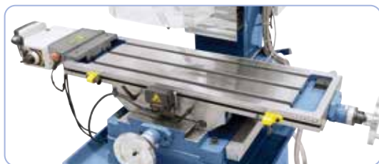
Large cross table with T-slots and coolant groove. Picture with optional available power feed AL 450 D.
