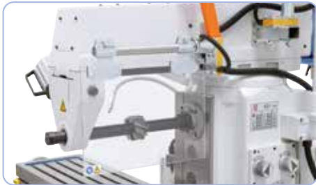
Serially equipped with counter bearing and long milling arbour, allowing horizontal milling.
