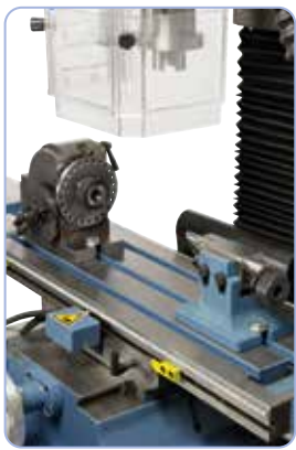
Semi-universal dividing head BS-0: ideal for machining of shafts.
