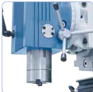
Large spindle (Ø 90 mm) guarantees high stability.
