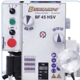
Digital display for drill depth increases comfort.
