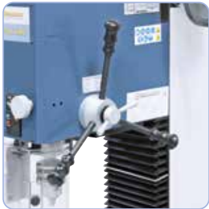
Large star handle allows easy spindle feed when drilling, handwheel allows fine adjustment when milling.
