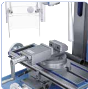
Milling with precision machine vise PS 75
