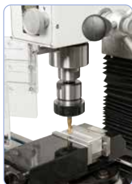
End milling The machine can be equipped with a tapping chuck set M5 - M12 for thread cutting.
