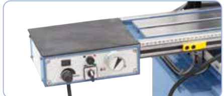
Serially with steplessly adjustable table feed for increased comfort FTV 6 (Art. no. 02-1032 / 02-1033B).
