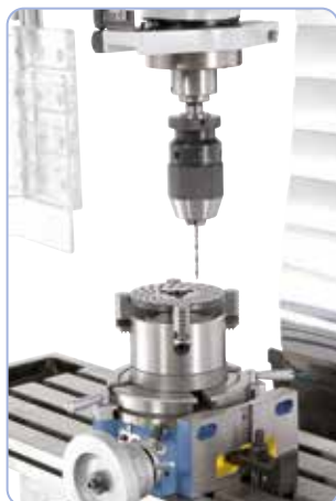
Drilling of coordinates
