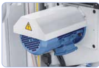
Positioning motor for table height adjustment (z-axis).
