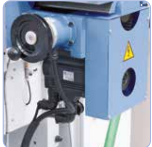
Electronic hand wheels for manual travel and 3 powerful servo motors in x-, y- and z-axis come standard.
