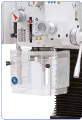
Height adjustable chuck guard and micro switch guarantees high safety standards
