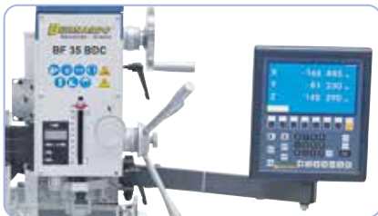
Digital readout Bernardo ES-12 V in x- and y-axis comes standard (Art. no. 02-1117).
