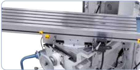
Milling table tilts from -45° to +45°.
