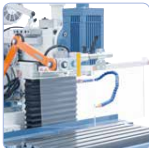
Adjustable protective cover, useable for vertical and horizontal milling works
