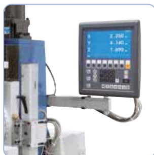
The digital readout in all three axis allows an increase in productivity of up to 50%.
