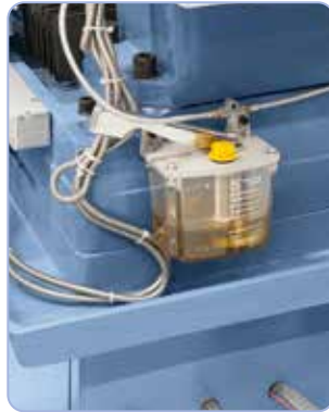
Central lubrication for all guideways come standard.
