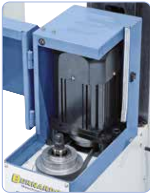
Balanced drive pulleys guarantees smooth running.
