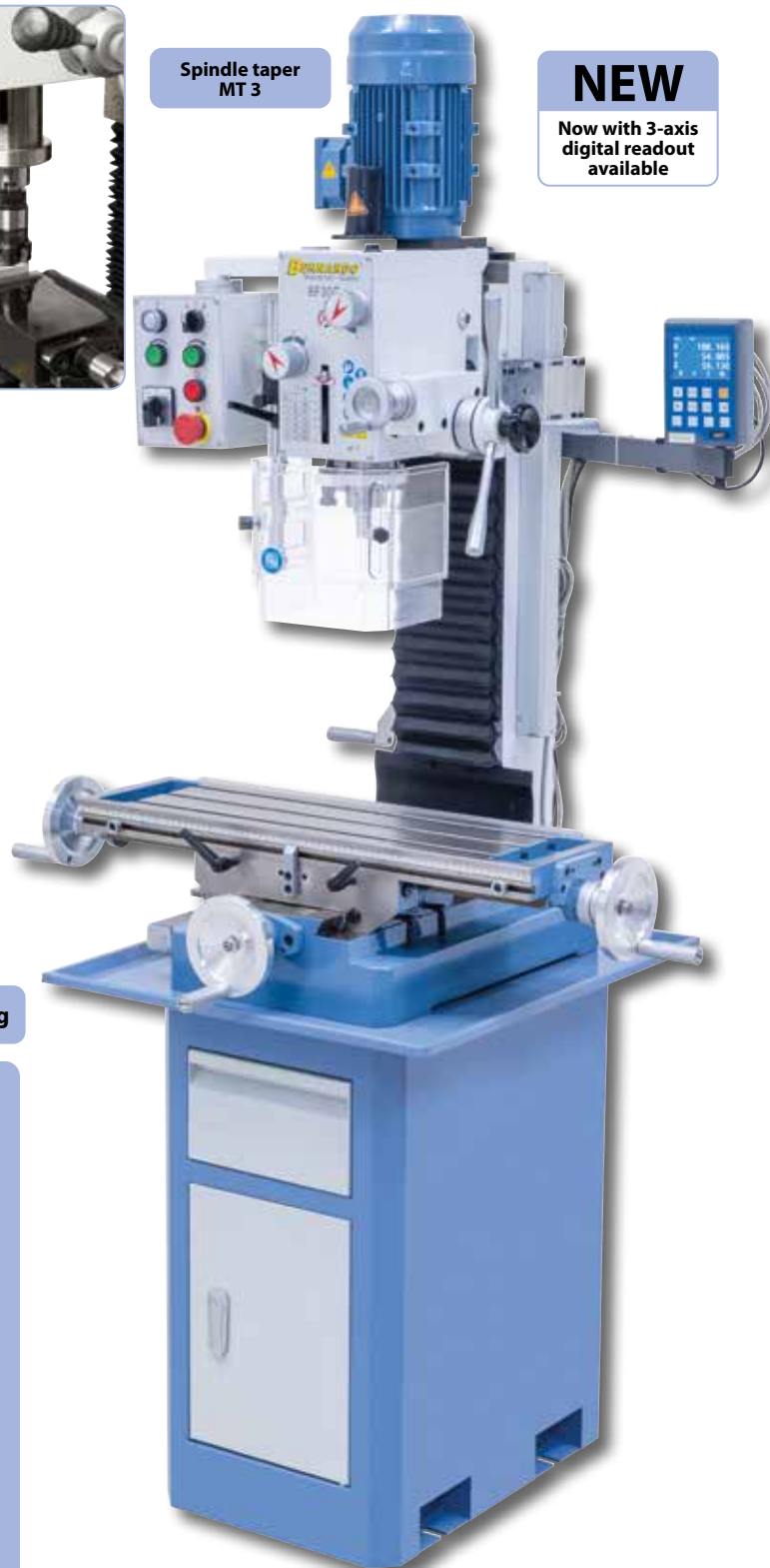
Powerful 2-step motor with 0,75 / 1,1 kW input power.
