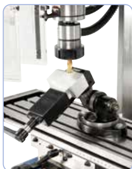
Milling with precision universal machine vise PGS 50.
