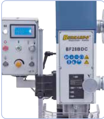
Digital speed and spindle stroke indicator included as standard equipment
