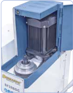
Balanced drive pulleys guarantees smooth running.
