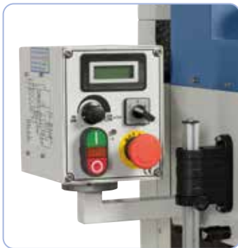
Digital speed display as well as left and right turning as standard.
