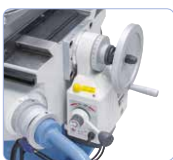
Positioning motor for table height adjustment (z-axis).
