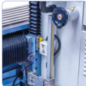
Electronic hand wheels for manual travel in x-, y- and z-axis come standard.
