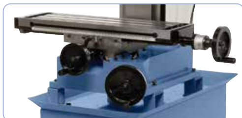
Handwheel, located on the front of the machine, makes height adjustment of mill head very user-friendly.
