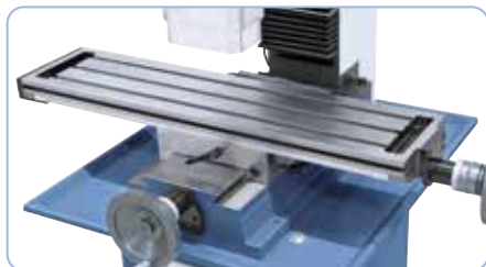
Surface treated cross table with 3 T-slots.
