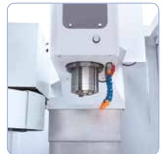
Robust headstock, tool change either manually or automatically
