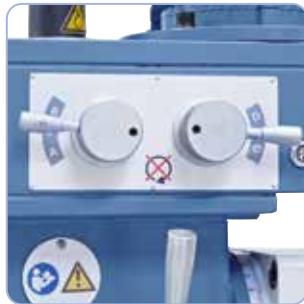
Clearly arranged, accessible control elements allow easy speed change.
