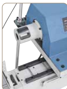
Precise roller guiding allows accurate movement of drill unit.
