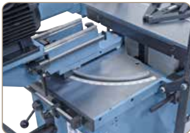
Drill head tilts 60° to right and left.
