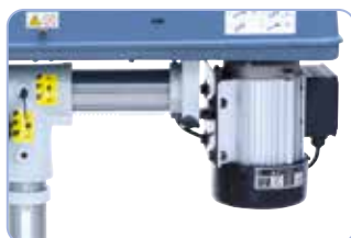
Powerful aluminium motor in accordance with the IP 54 standard.
