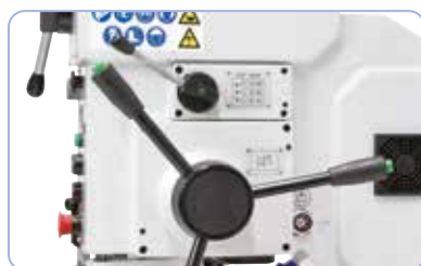
Drill feed made manually or by electromagnetic clutch
