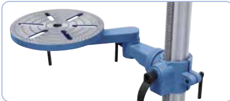
Work table swivel 360° which is ideal for coordinate drilling.
