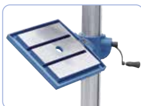
Drill table can be tilted from -45° to +45° and can be turned 360° around the column.
