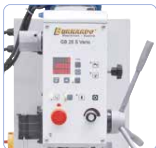
Intermediate transmission system allows for easy gear settings. Speed selection by potentiometer.
