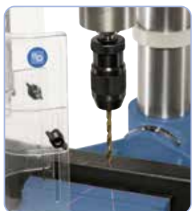
Complete with cross line laser device to achieve high accuracy.
