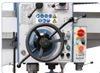
3-way spindle feed: lever allows quick adjustment, handwheel allows fine feed or automatic feed
