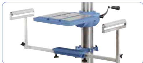
An extendable drill support can be added to stabilize long workpieces.
