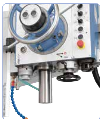
Speed/ feed adjustment situated on underside of drill head.
