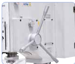
The drill feed takes place manual or electro-magnetic clutch
