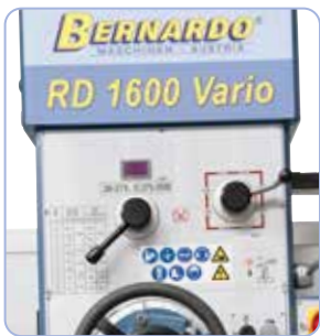
Speed and feed settings are on front of drill head.
