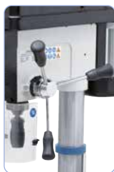
Ergonomically arranged handles allow for easy spindle feed.
