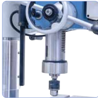
Big dimensioned spindle with 140 mm stroke.
