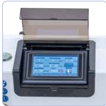
Comfortable work: adjustment of the thread size, pitch, speed and drill depth directly over the integrated touchscreen.
