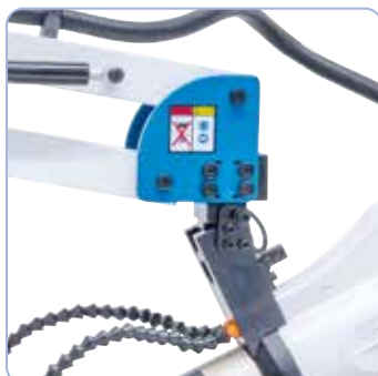
Including swivel unit for horizontal or inclined cutting.
