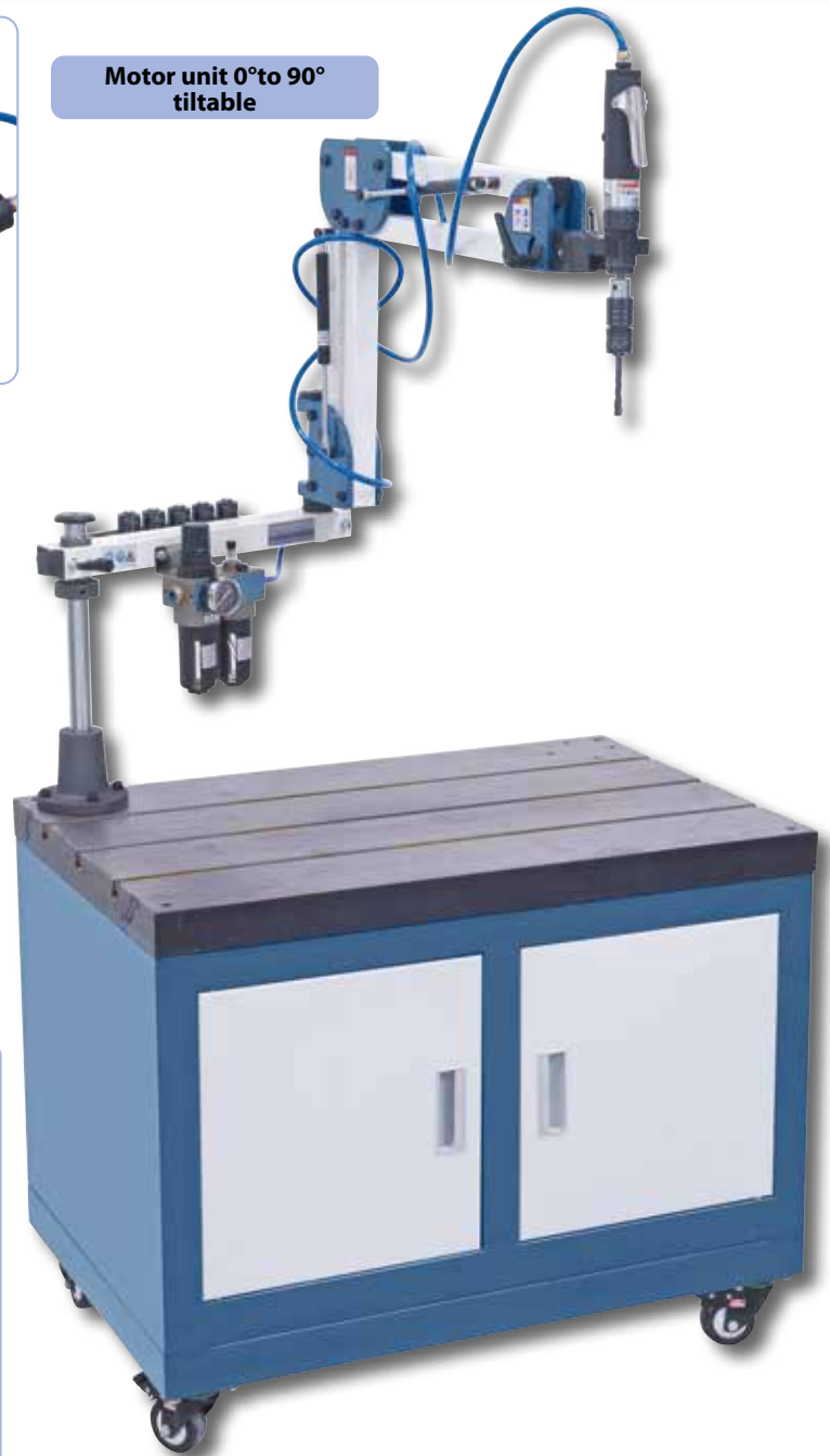
Including swivel unit for horizontal or inclined cutting.
