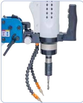
Micro-spray system and blow-out device comes standard
