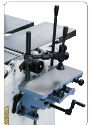
Mortising unit comes complete with large support table and eccentric clamp.
