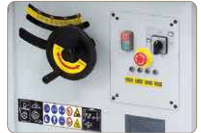
User-friendly arranged switches and control elements, electronic speed display via LED.
