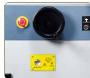
Handwheel ensures quick and easy height adjustment of milling spindle, easy to read with magnifier.
