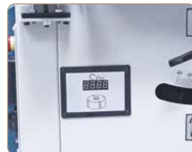
Electronic display of spindle speed settings.
