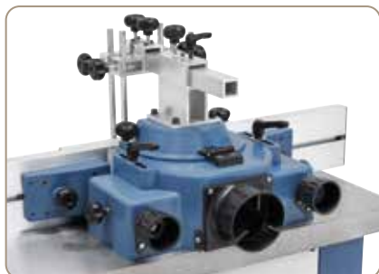
The solid moulding fence can be adjusted for tools up to 200 mm. Stop bars on both sides feature fine adjustment.
