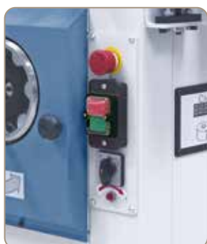
The electronic control elements are ergonomically arranged at the front of the machine.
