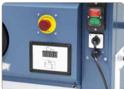
Electronic display of spindle speed settings.
