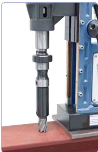
Core drilling with cutter extension
