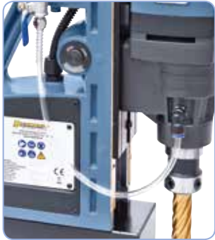
Automatic internal lubrication, coolant fluid goes straight to tip of core drill
