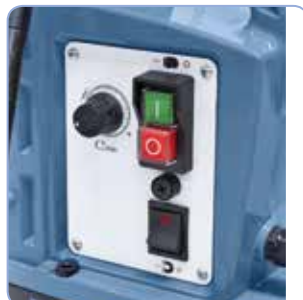
Exact adjustment of the cutting speed using a potentiometer.
