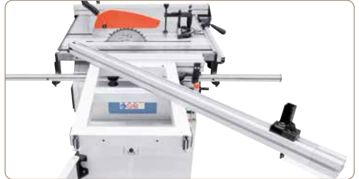
The steplessly tiltable telescopic fence (2 x 45°) can be mounted at the front or rear of the square table.
