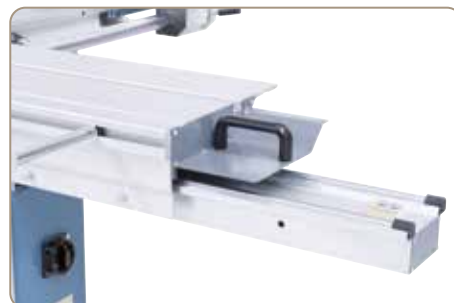
Torsion-free aluminium sliding table features smooth guiding to guarantee precise working.
