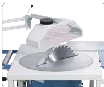
The protective cover follows the sawblade movement.
