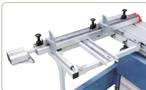
Square table can be moved along the entire sliding table length and taken off at any position. The telescopic fence, featuring 2 solid tiltable stops, allows precise adjustments.
