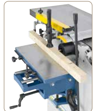
The mortising unit is ideal for drilling deep holes, dowels and oblique holes etc.
