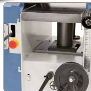
Thicknessing table with center column and support ensure accurate planing.
