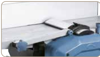
Cutterblock cover according to CE standards.
