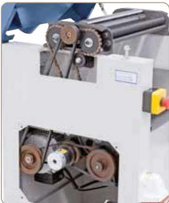
The infeed is driven by a solid chain drive. The infeed speed is 5 - 7 m/min.
