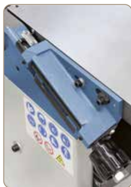
Quick and easy adjustment of chip removal.
