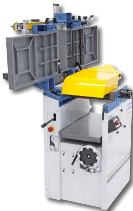
The solid planing unit features a precisely bedded spiral cutter head to guarantee best results.
