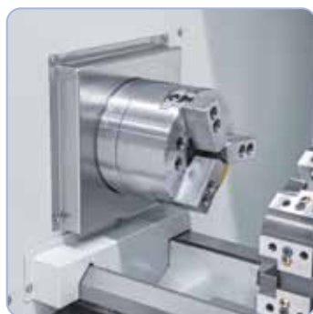
Hydraulisk 3-bakket patron diam. 200 mm
