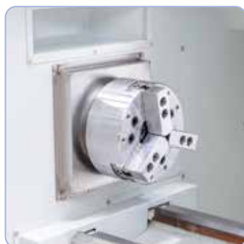
Hydraulisk 3-bakket patron diam. 200 mm
